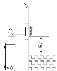
Figure 16 - Square Termination Clearance at Ground Floor Installation
